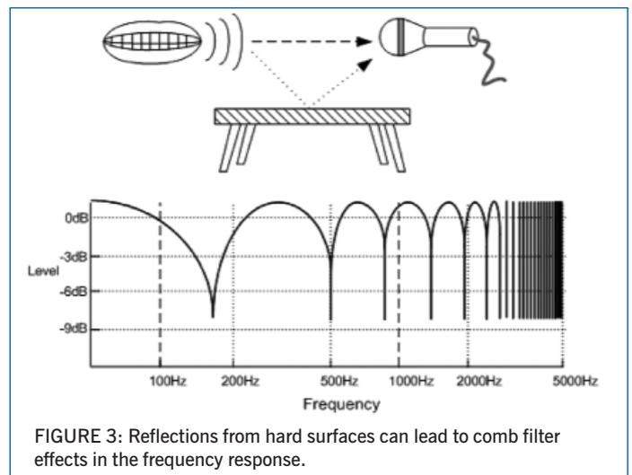
FIGURE 3: Reflections from hard surfaces can lead to comb filter effects in the frequency response.
