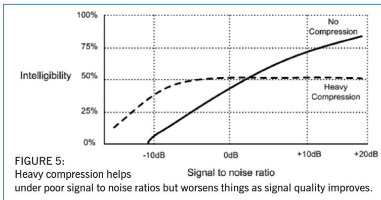
**FIGURE 5:** Heavy compression helps under poor signal to noise ratios but worsens things as signal quality improves.
